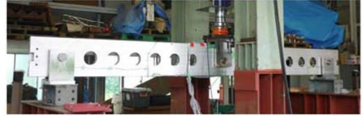
・ Main frame :23ton of maximum loading capacity
