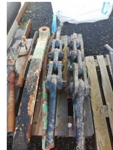
Fig 2 Detail showing the placement of the 3ft bars, with the 1902 chain along the top.
