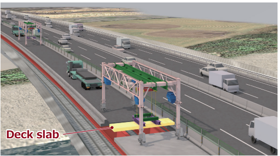
* Conceptual image of multiple-section deck slab replacement at Tomei Tamagawa Bridge
