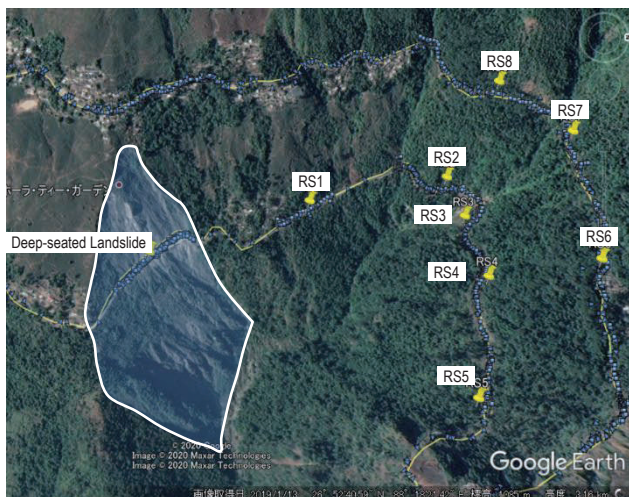
Figure 5 Deep-seated Landslide and Road Sinking in Paglajhora
