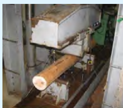
支点間隔800mm, 載荷点間隔200mm
