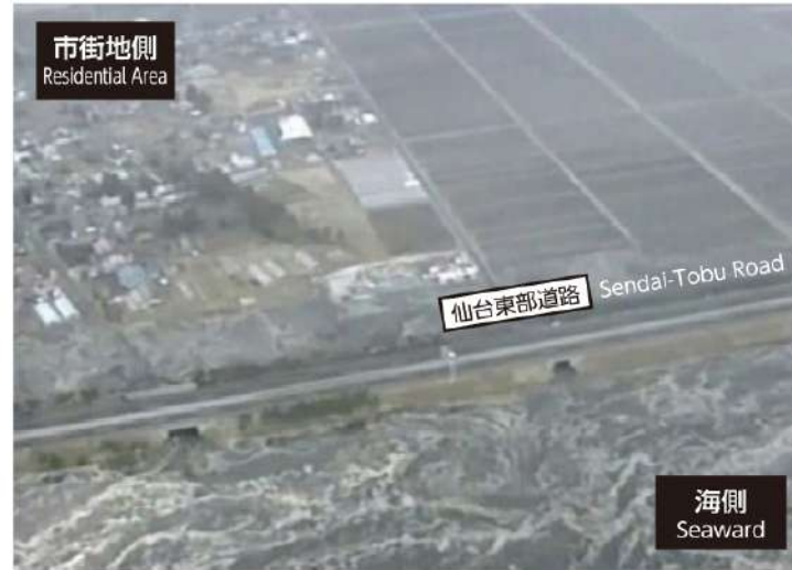
仙台東部道路が内陸の市街地への津波・がれきの流入を抑制 The Sendai-Tobu Road blocked the tsunami and rubble from reaching farther inland.
