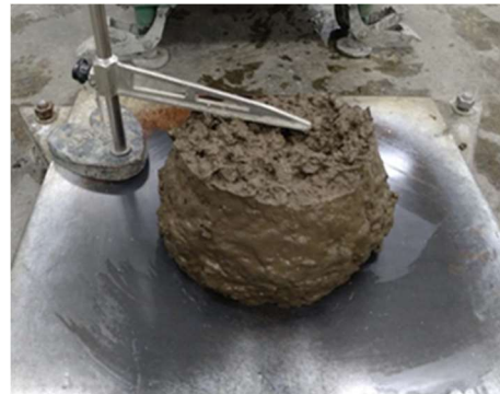
Slump property of LigninCrete
