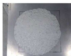
Slump flow of 60 cm
