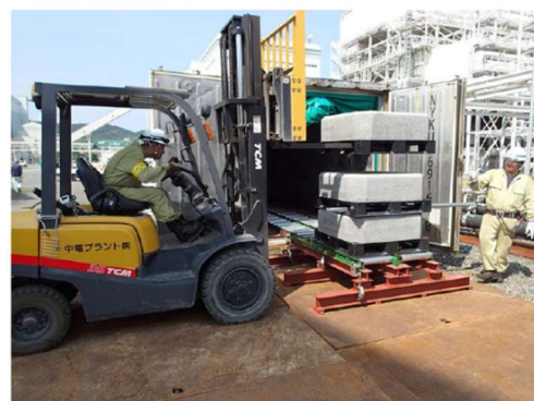
Figure 1.2 Loading CO 2 -SUICOM concrete products into the carbonation curing tank
