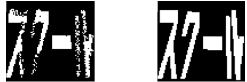
Fig. 5 Examples of the thresholding results (left: original image; right: segmentation result).
