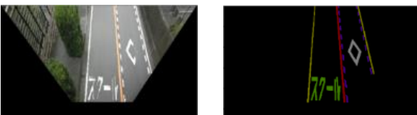
Fig. 3 Examples of the obtained BEV images (left: original image; right: segmentation result).
