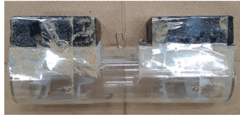
Added weight (578 g = 8 times of pipe weight)
