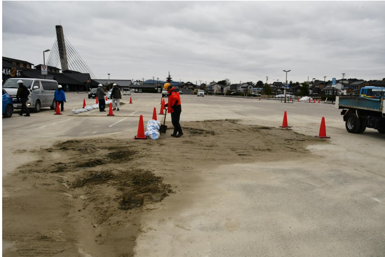
Ejected sand due to liquefaction on flat ground (Map①)
