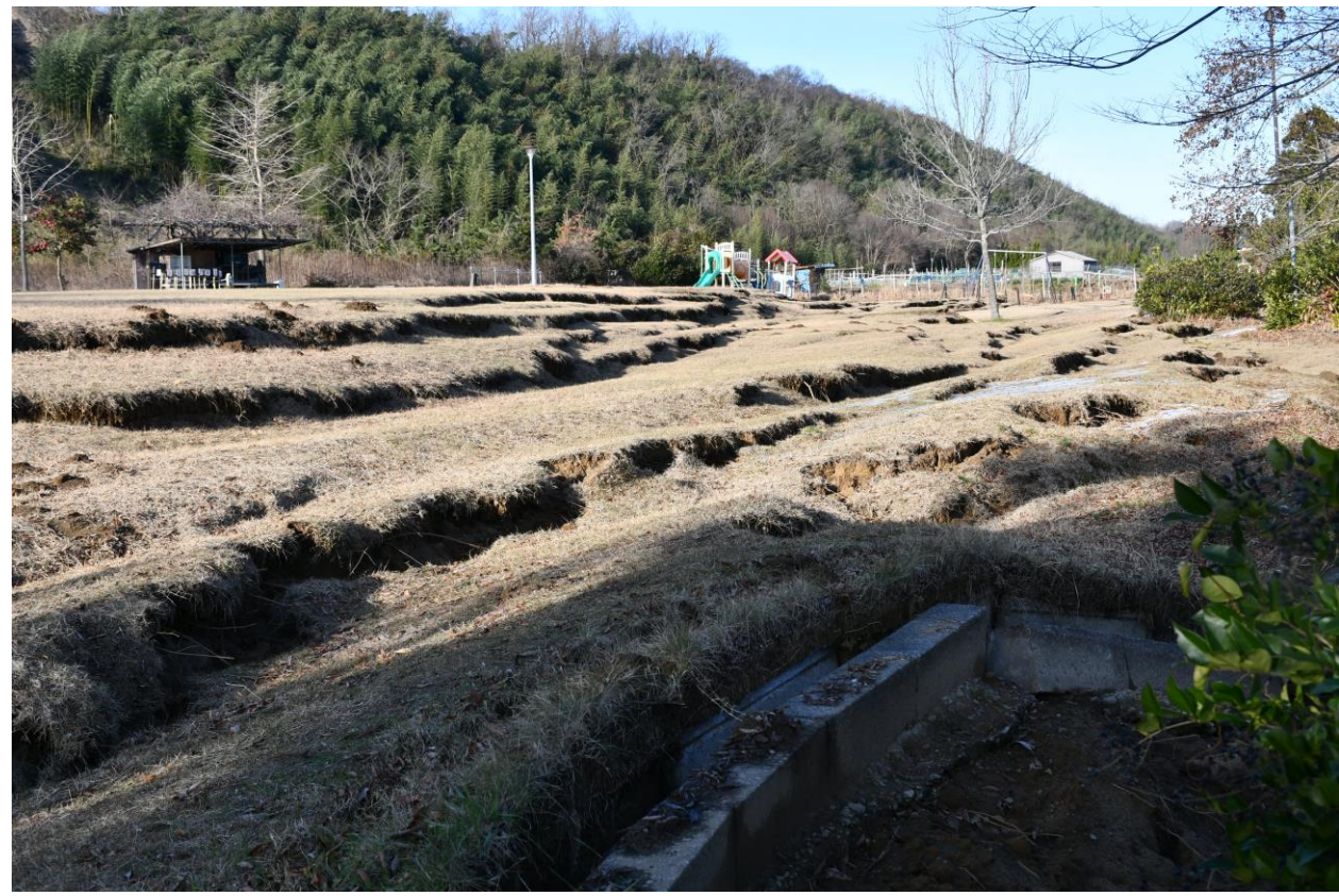
Ground deformation due to lateral flow (Map①)
