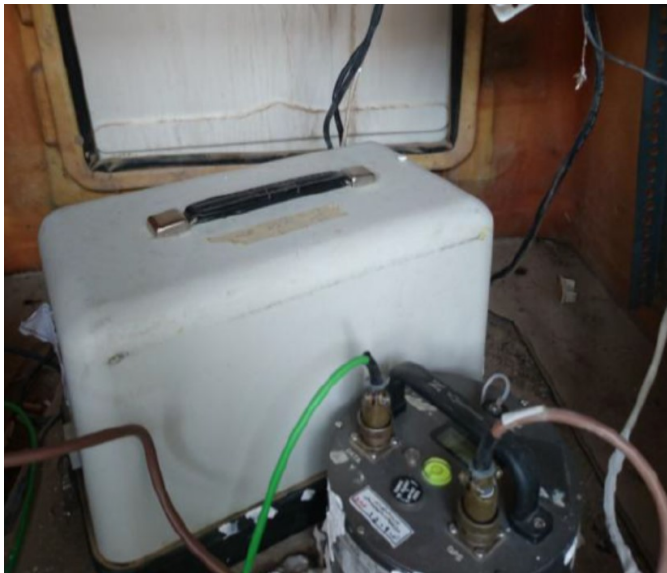
SSA-2 permanent instrument along with the temporary CMG5TD instrument (source: BHRC)
