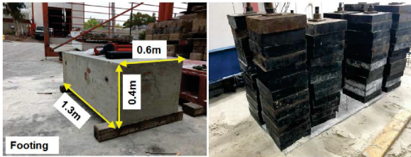
Fig. 2: Model footing prior to placement and weights to replicate target contact pressure
