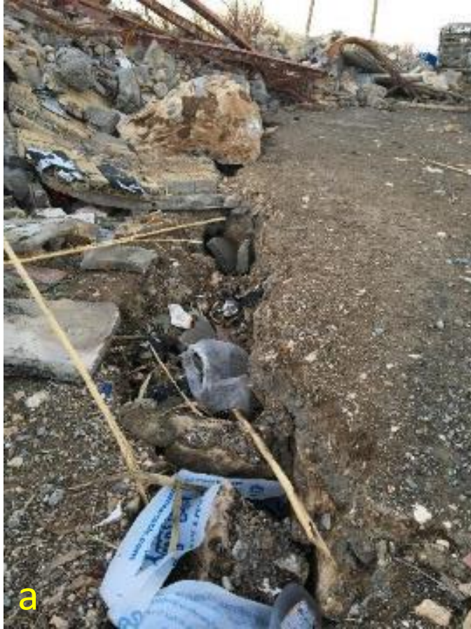
Fig. 12 (a & b) Soil rupture in Palan-e Olya village
