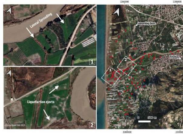
Figure 11. Liquefaction and lateral spreading sites at the coastal plain south of Antakya. Most of the sites are found along the course of Asi (Orontes) river and over abandoned fluvial features.
