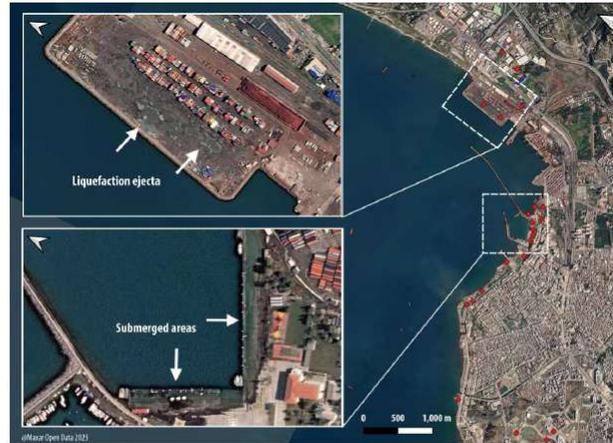
Figure 12. Liquefaction and lateral spreading sites at the port city of Iskenderun. Most of the sites were found along the coastal front and within the reclaimed port facilities and piers of the old port. Insets show liquefaction ejecta and submerged sections of piers. Widespread lateral spreading and subsidence was manifested along a > 6km section of the coastal front.
