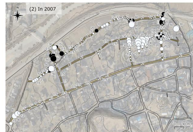
Fig. 3 Pavement fractures observed in Toge Villag in: (1) 2024, and (2) 2007: Open circles and solid circles with numbers in mm show tensile and compressional failure widths.
