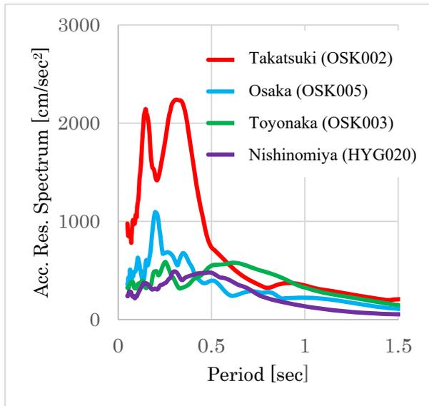
**Fig.2** Response spectra of four cities for the Osaka-Fu Hokubu earthquake
