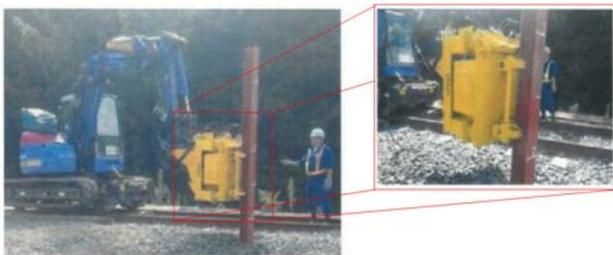
Fig.30 Situation of compacting use of the improved backhoe (from JR West)
