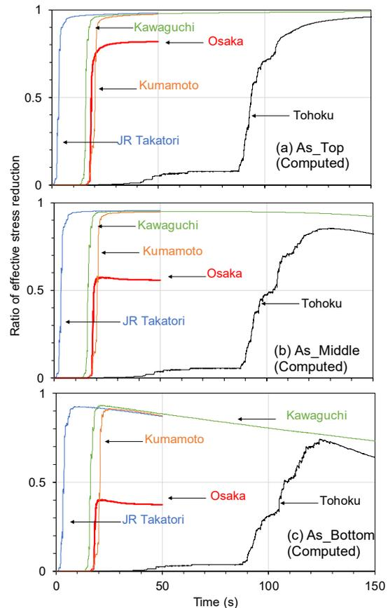
**Fig.16** Time histories of the effective stress reduction ratio of the liquefiable layer (As layer): (a) top of the “As” layer, (b) middle, (c) bottom
