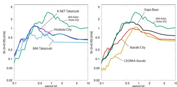
Fig.9 Velocity response spectrum (damping ratio of 5%)
