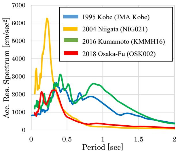
**Fig.3** Comparison of response spectra of past earthquakes
