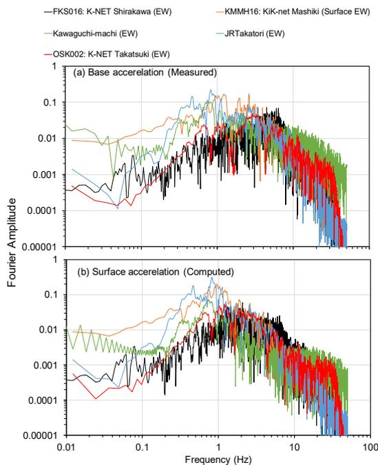
**Fig.15** Fourier amplitude spectrum of acceleration: (a) input (measured record), (b) response at the ground surface (computed)
