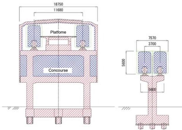
**Fig.25** Infrastructure (red) and transport section (blue) on Osaka Monorail
