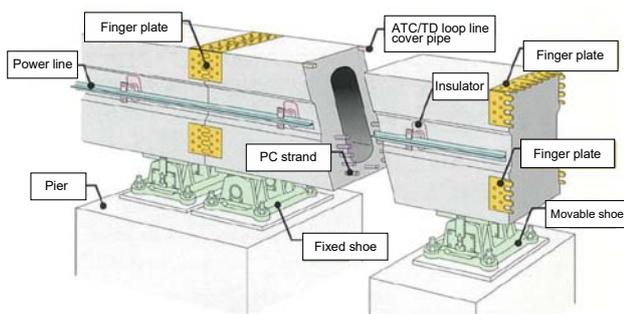
**Fig.26** Configuration of the PC rail girder (from Osaka Monorail)
