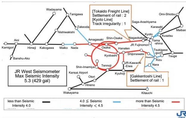
Fig.29 Damage to the JR West local line facilities (from JR West)
