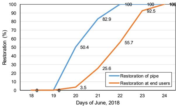
**Fig.21** Osaka Gas restoration process (restoration number 111,951 households)
