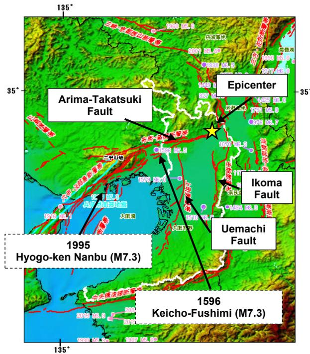
**Fig.1** Active faults in the Kinki region and large historical earthquakes (processed from reference<sup>3)</sup>)
