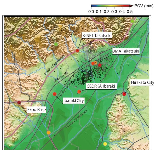
**Fig.5** Seismic observation point near the source and horizontal peak velocity. The black dots show the distribution of aftershocks for the day following the mainshock.
