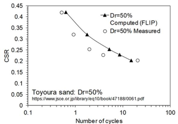
**Fig.13** Measured and computed liquefaction strength curves of Toyoura sand with a relative density of 50%
