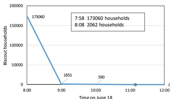
**Fig.24** Electric power recovery process (maximum blackout number = 173,060 households) (from Kansai Electric Power Co.)
