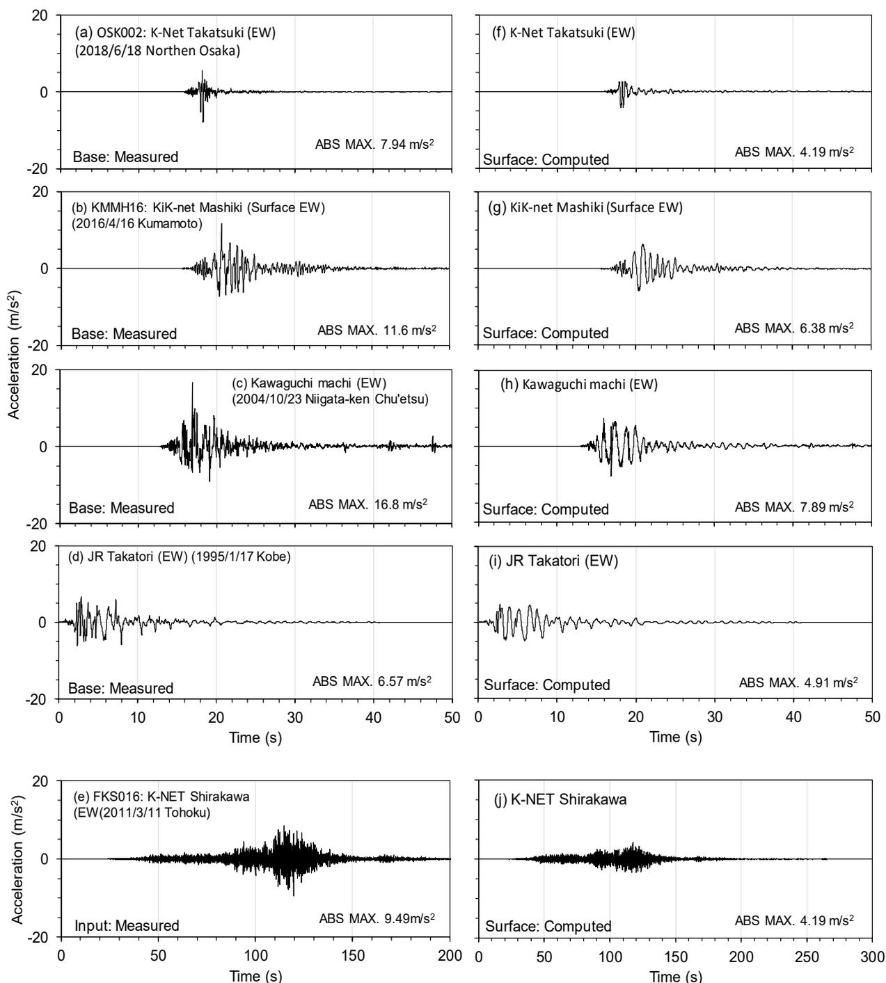
**Fig.14** Acceleration time histories of ground motions: (a)–(e) measured input motions; (f)–(j) computed surface responses
