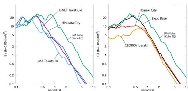
Fig.8 Acceleration response spectrum (damping ratio of 5%)
