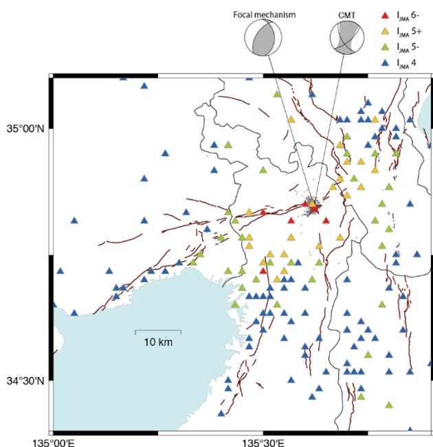
**Fig.4** Distribution of the epicenter, focal mechanism, and seismic intensity of the Osaka-Fu Hokubu earthquake. The red lines show the surface trace of the active fault<sup>6)</sup> and the gray dots shows the distribution of aftershocks the following day
