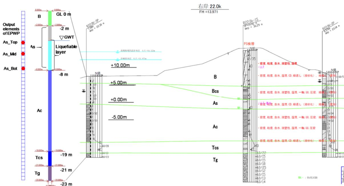
**Fig.12** Soil profile at the location near the 22 kilopost: borehole logs of the levee of the Yodogawa, and the finite element mesh after 13).
