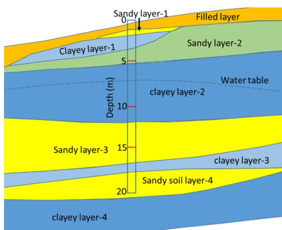
**Fig. 3** Soil profile estimated from borehole data (provided by JICA<sup>4)</sup>)
