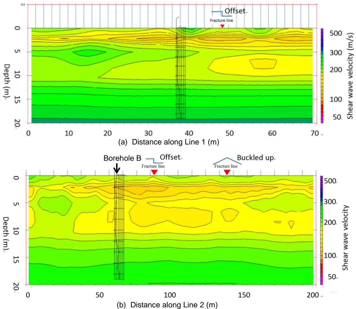
Fig. 6 Estimated soil profiles along Lines 1 and 2
