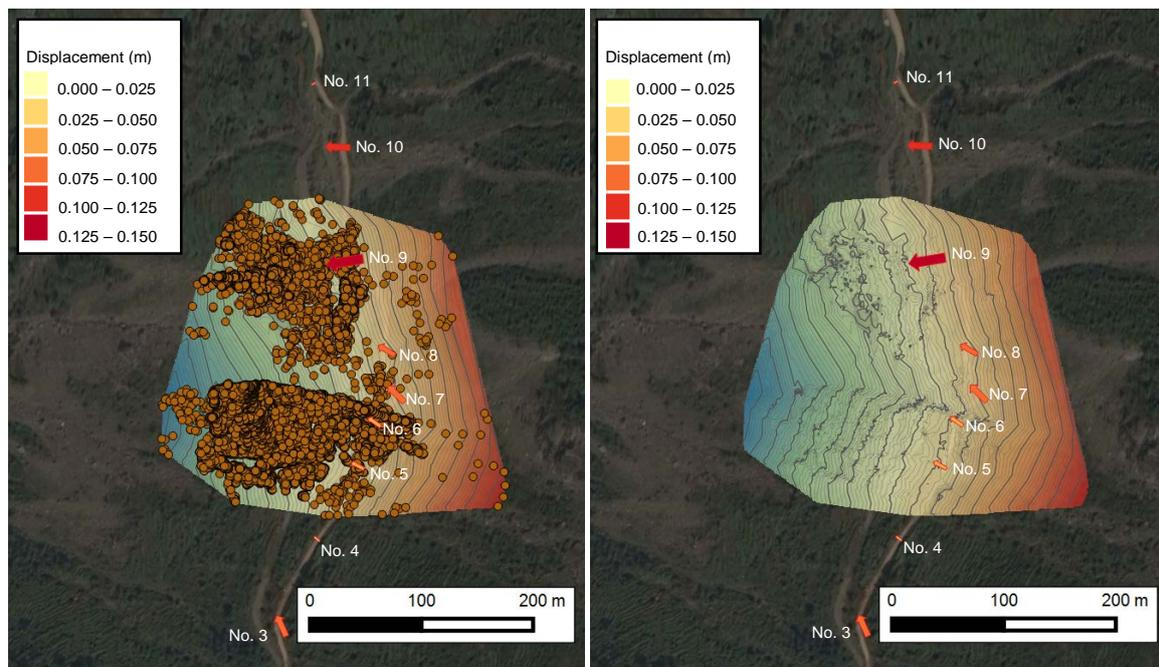
**Fig. 12** Micro terrain model (right) for a fraction of the creeping slope extracted from photos: Stereo-photogrammetry software allows to detect dots on the left figure automatically/ manually from photos for creating the 3D image shown on the right figure. (Photos from Google Earth)
