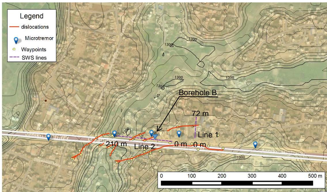
**Fig. 4** Surface wave Survey test profile lines 1 and 2
