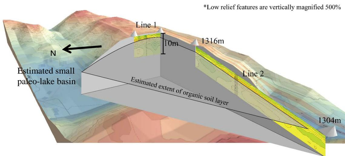
**Fig. 8** Birds eye view of the damage section with observation points and SWS test profile
