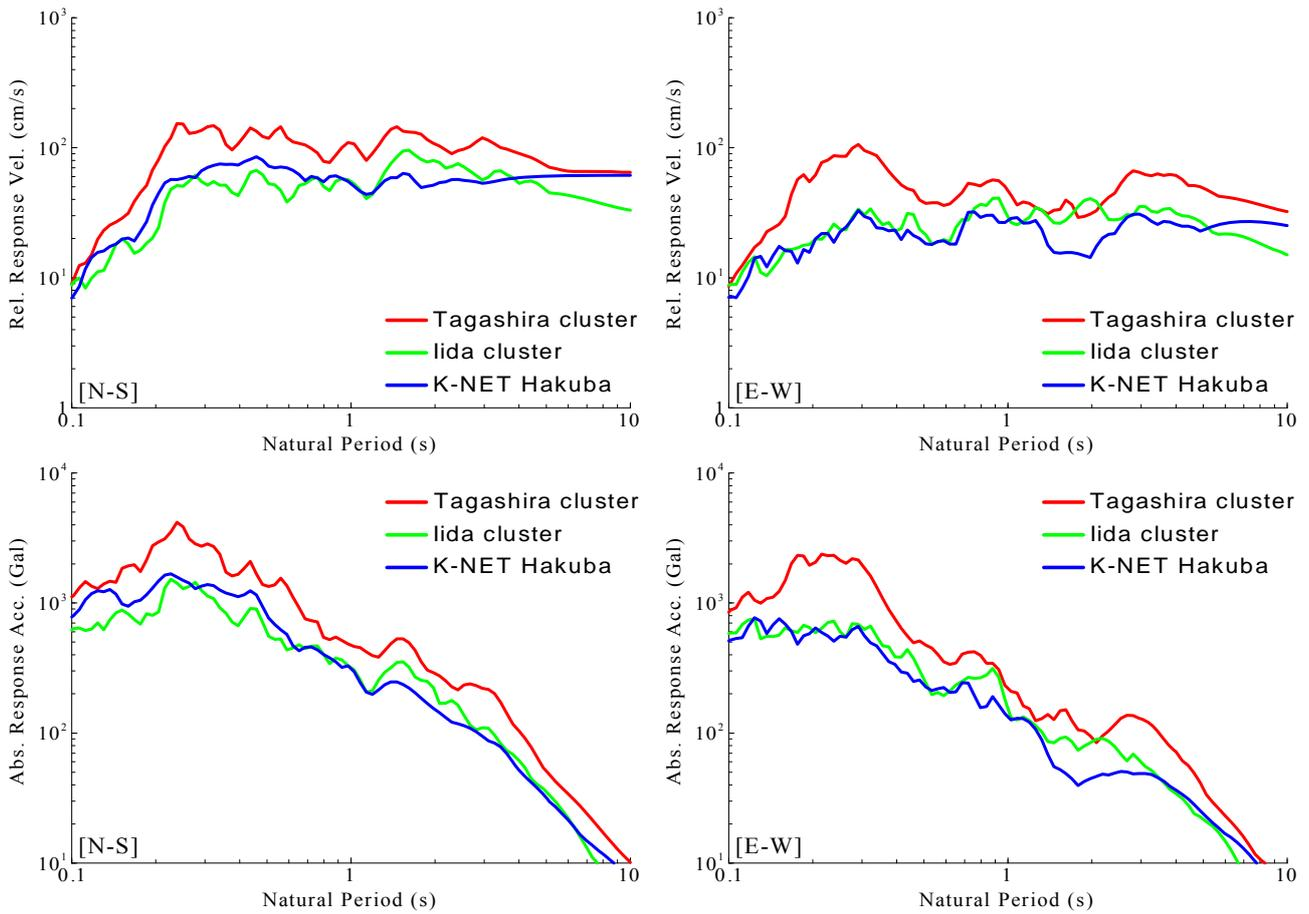
**Fig.19** The estimated response spectra at the sites of interest with the observed response spectra at K-NET Hakuba site.
