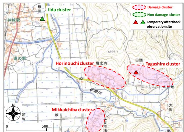
Fig.4 Damage and non-damage cluster in Kamishiro Area.
