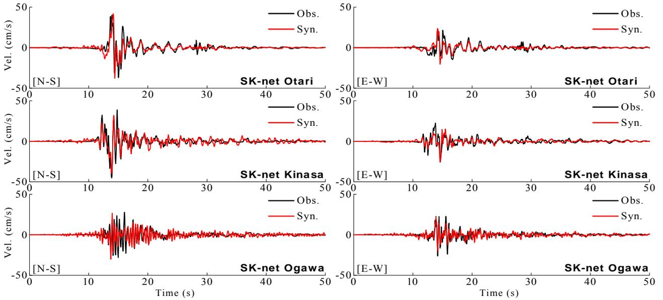
**Fig.14** Confirmation of the the site-effect substitution method using the observed seismic waveforms.
