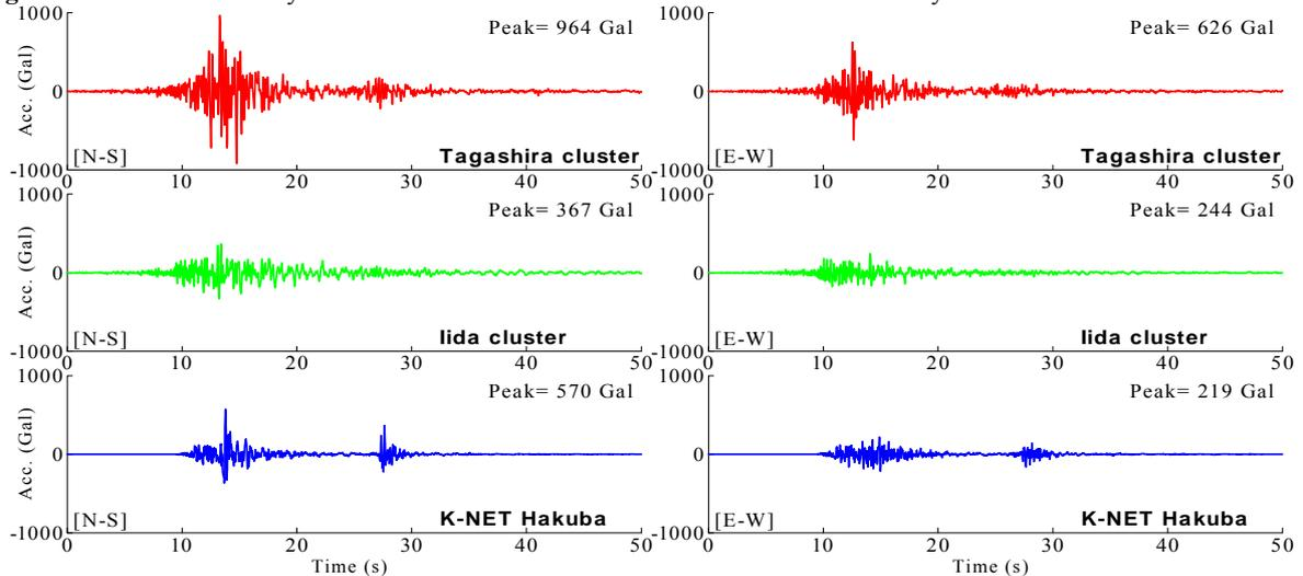
**Fig.18** The estimated acceleration waveforms at the sites of interest with the observed acceleration waveforms at K-NET Hakuba site.
