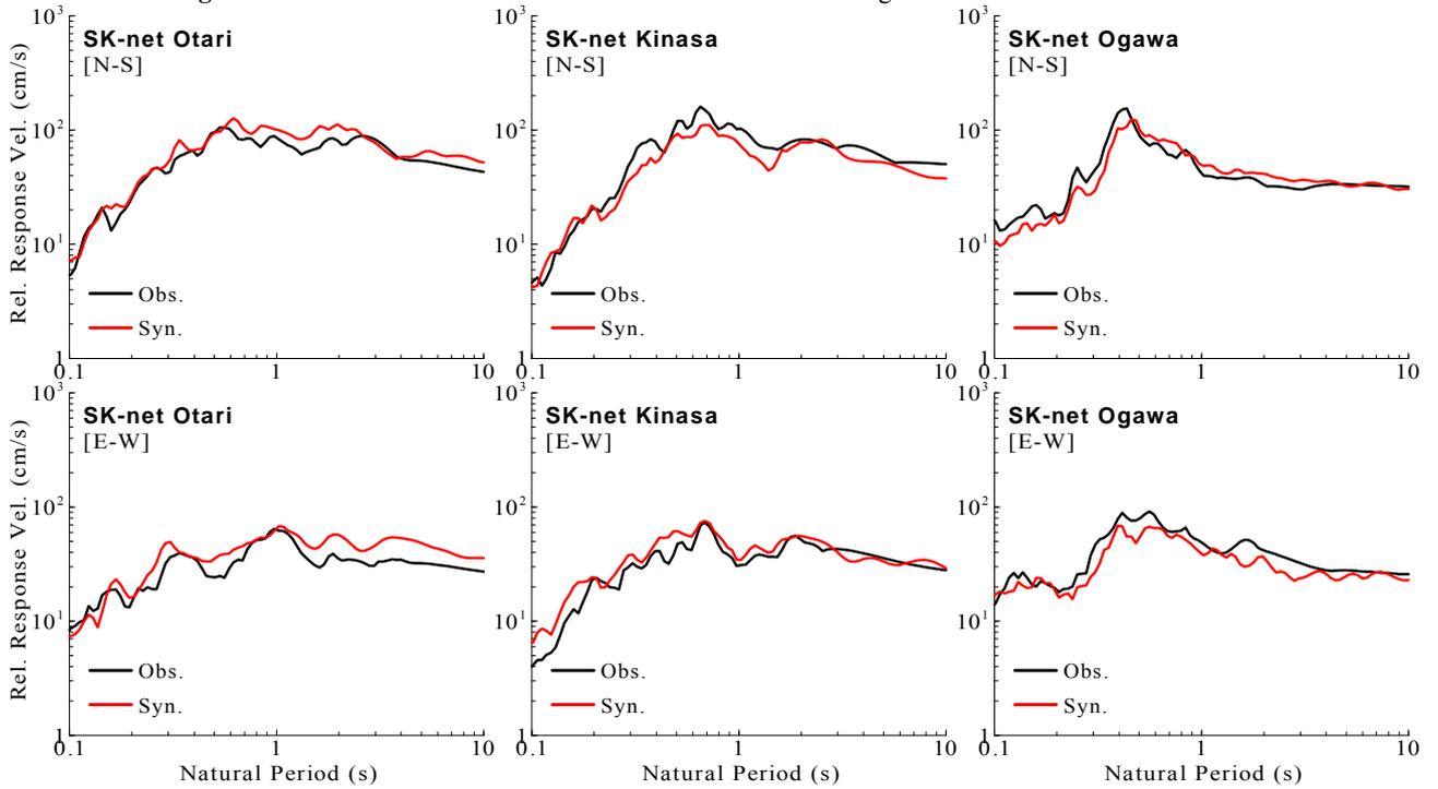
**Fig.15** Confirmation of the the site-effect substitution method using the observed velocity response spectra.
