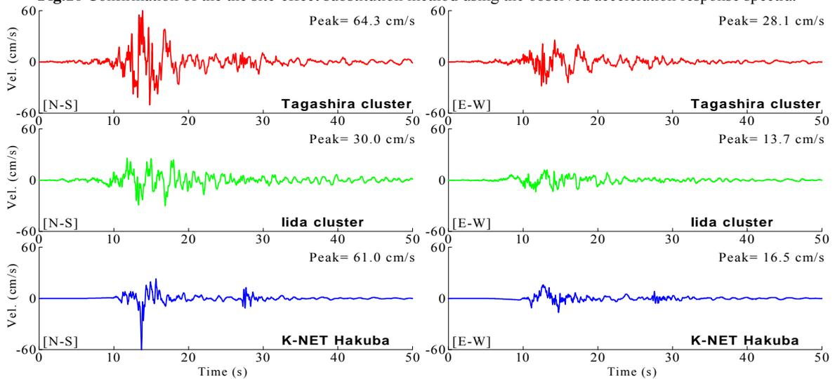
**Fig.17** The estimated velocity waveforms at the sites of interest with the observed velocity waveforms at K-NET Hakuba site.
