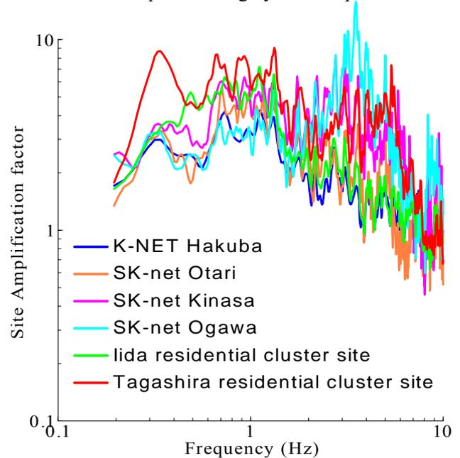
Fig.10 Comparison of site amplification factors.
