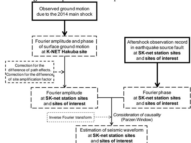
Fig.11 Framework of site-effect substitution method.
