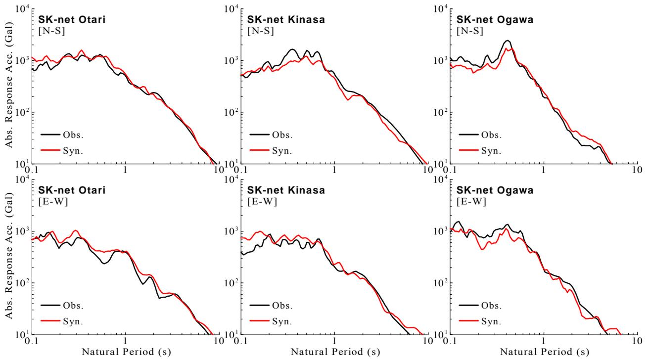
**Fig.16** Confirmation of the the site-effect substitution method using the observed acceleration response spectra.
