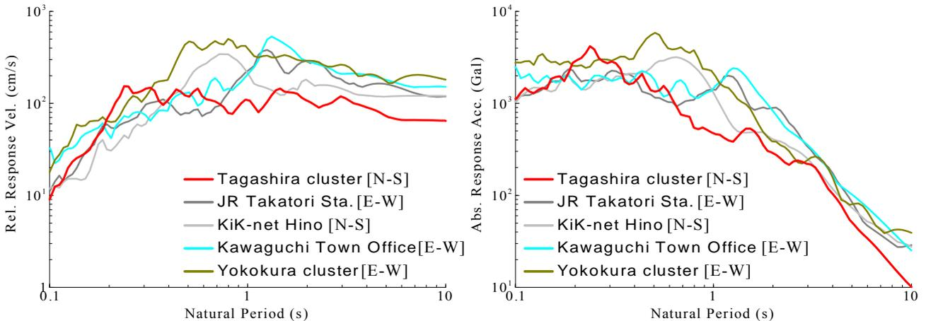
**Fig.20** The estimated response spectra at Tagashira residential cluster site with the response spectra due to the large scale earthquakes.
