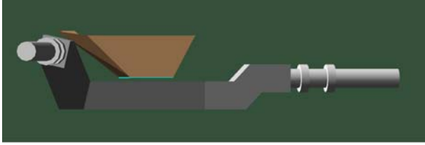
Fig. 5 Three-dimensional illustration of under-crossing concrete encased structure.
