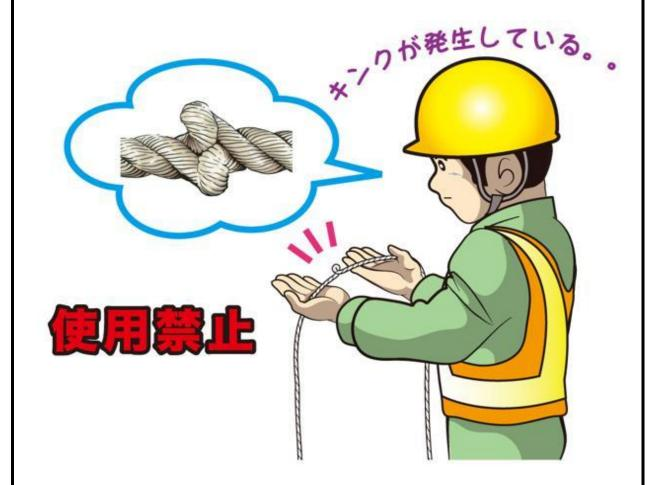
If a kink occurs in a wire rope used for lifting work, its strength is reduced even if the kink has been removed.
