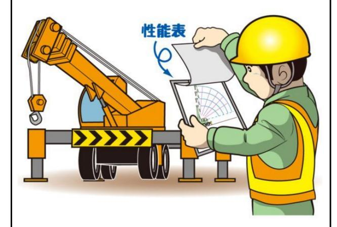
In lifting operations using a crane, check in advance the lifting capacity of the crane using a performance table. It is important to always carry out the work based on a safe work plan.
