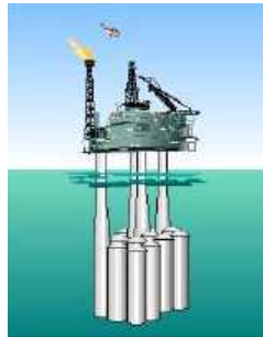
Condeep (abbr. concrete deep water structure )
