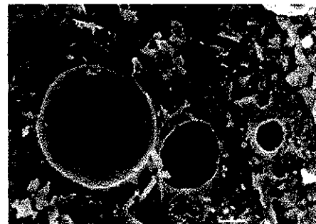
Figure 2. Microstructure of a high performance concrete: low porosity and homogeneity of the matrix [2]
