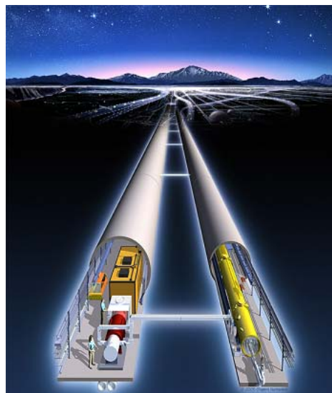
Figure 1 : Conceptual Rendering of Linear Collider (courtesy of KEK: High Energy Accelerator Research Organization)
