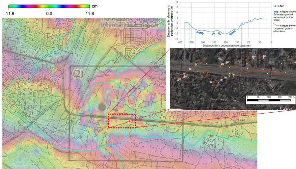
Fig. 12 Disturbance of InSAR fringe pattern near sagging section of Araniko Highway
