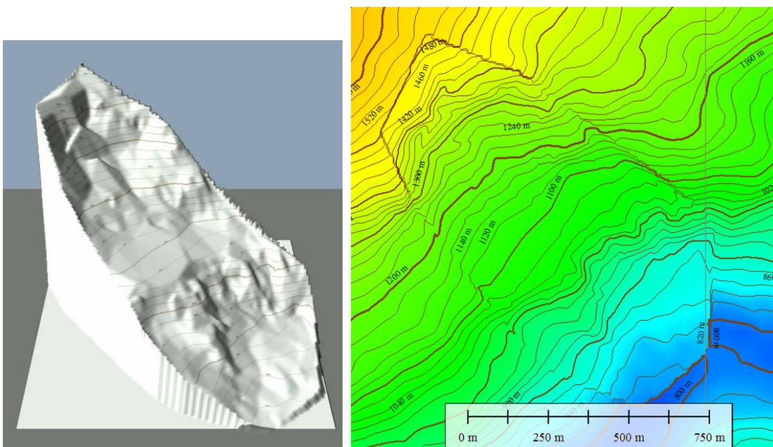
Fig. 5 DEM of slip surface of Sunkoshi Landslide
