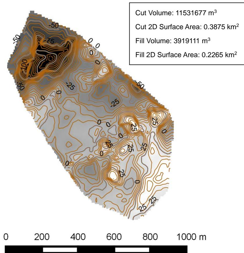
Fig. 6 Change in elevations within the exposed slip surface
