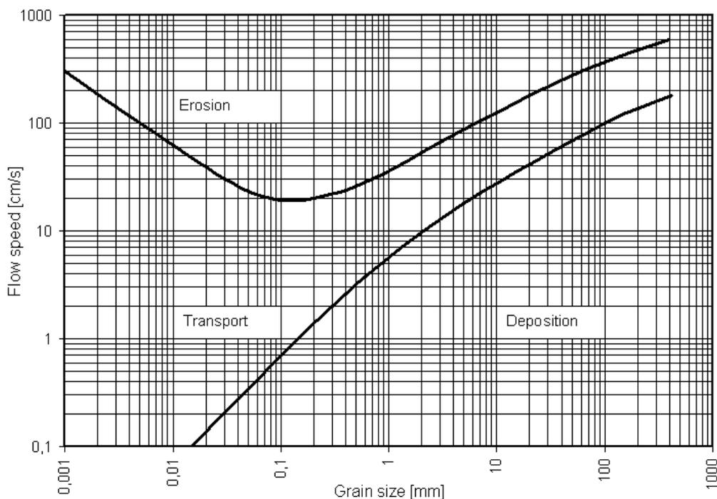
Fig. 3 Hjulström curve showing the critical current velocity required to move grains on a plane bed
