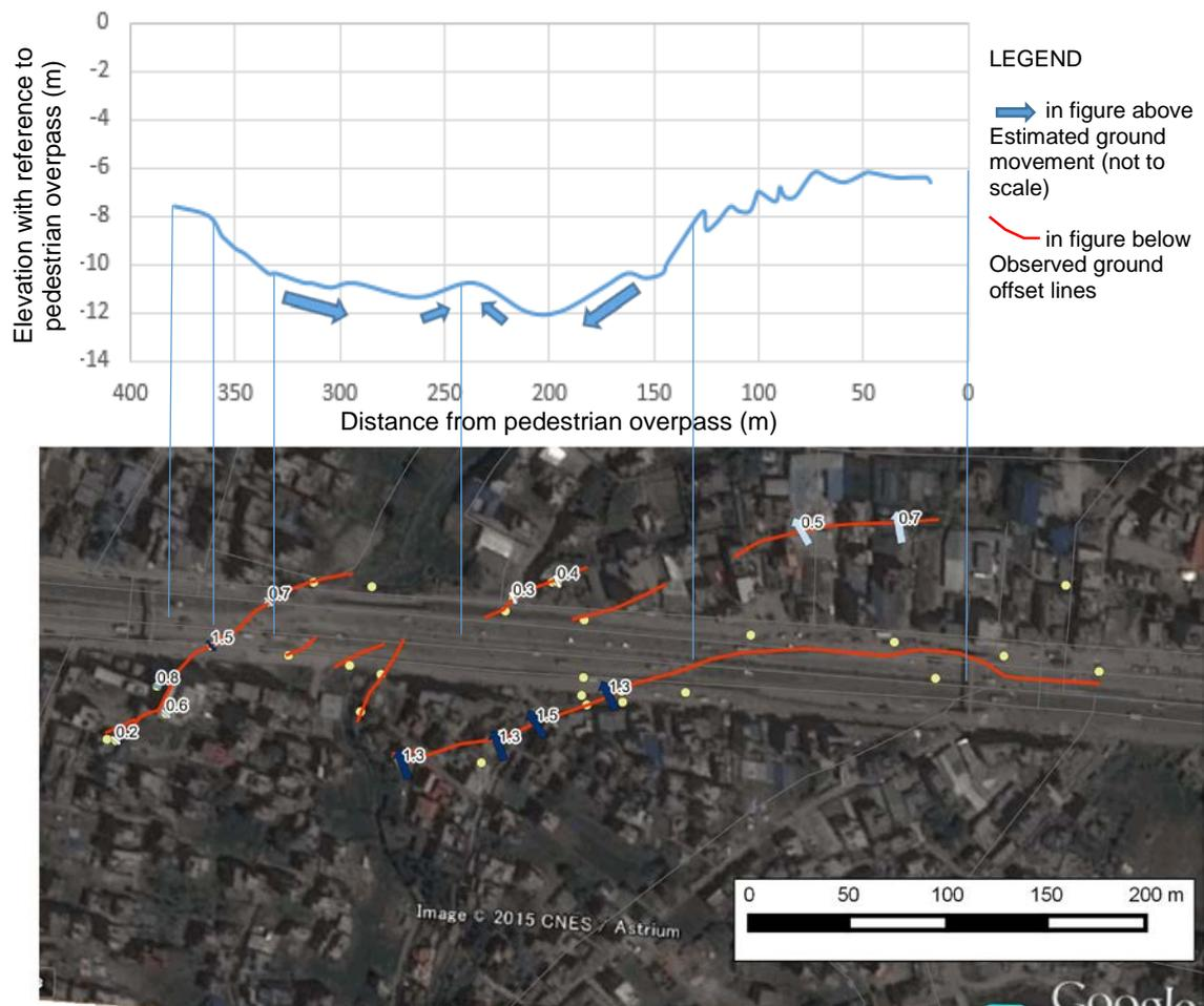
Fig. 10 Depressed section of Araniko Highway and ground offsets (Photo from Google Earth)
