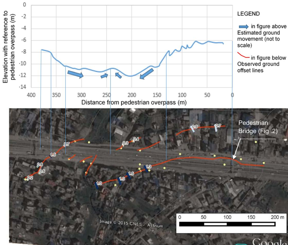
Fig. 1 Depressed section of Araniko Highway and ground offsets<sup>3)</sup> (Photo from Google Earth)
